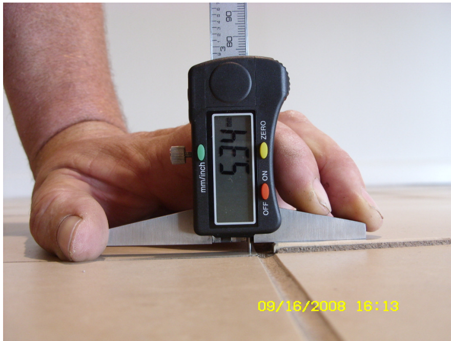
Precise measurement of tile lippage with digital offset depth gauge
