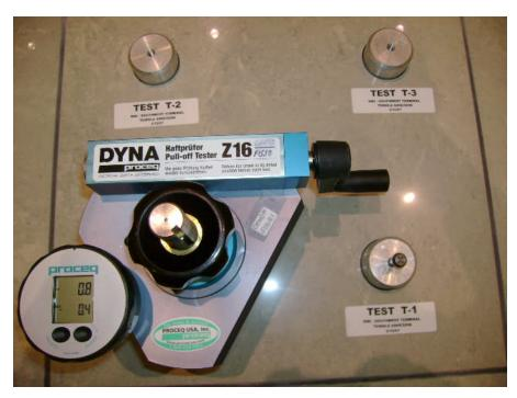
PROCON utilizes precision digital hydraulic load testing equipment
