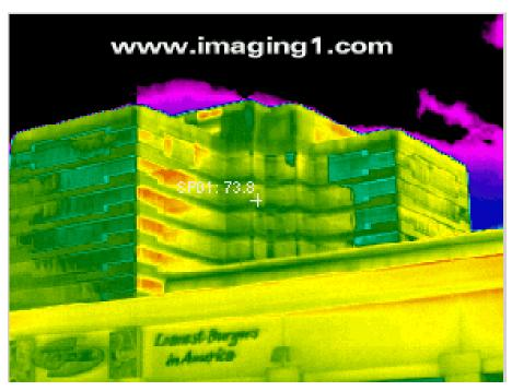
Thermoscan reveals heat loss and air exfiltration around the structural frame and through the building envelope resulting from failure to properly install insulation and / or water infiltration
