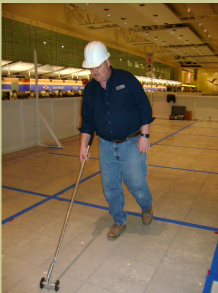
PROCON utilizes efficient rotary percussive acoustic sounding equipment
